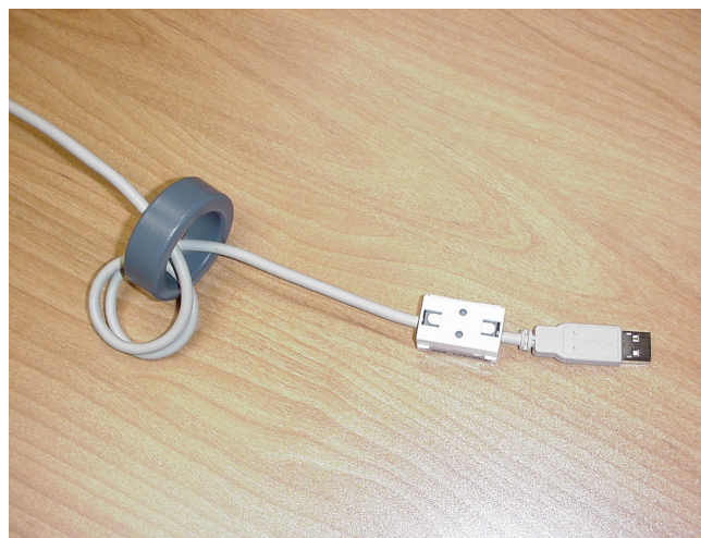
Figure 7 - Example of a USB Cable Using Ferrites
