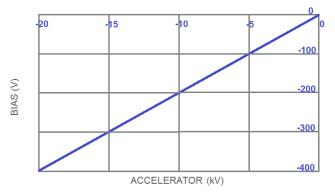
An Accelerator output of 20kV will generate a current of 40uA feedback into the 500M feedback resistor, which is equal to a voltage of 400V generated across the 10M $\Omega$  resistor. So the Bias sits at -20400V which blocks the flow of electrons. A positive voltage on the Bias reduces the HV and allows current to flow.
