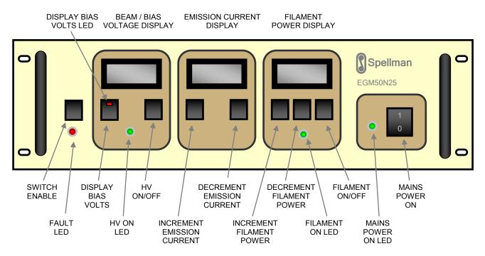
Figure 3 – Front Panel Features
