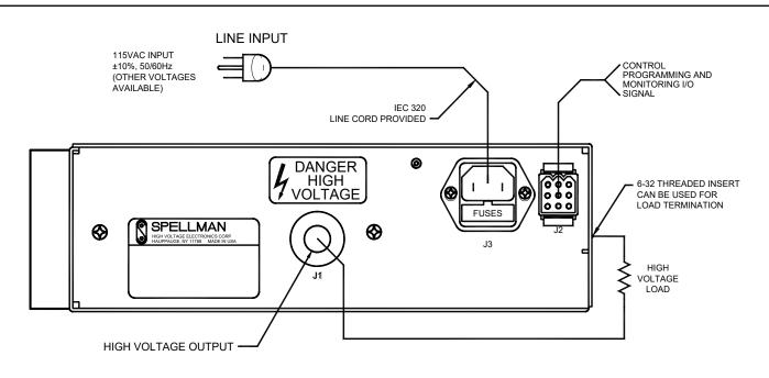
Figure 3.1 Typical Operating Set Up
