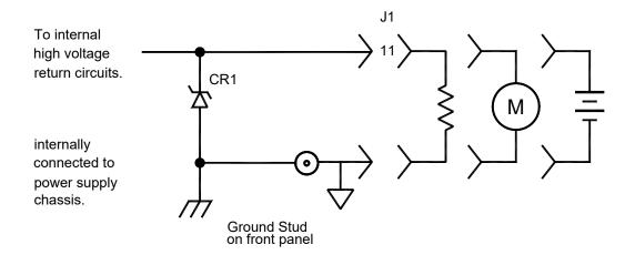
Figure 5.1 Floating Ground Interface Circuit
