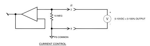
Figure 3.2A Remote Programming Via Voltage Source
