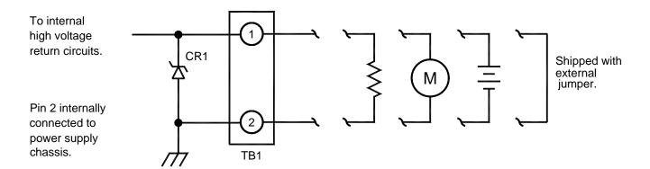
CR1- Polarity dependent on output voltage polarity. Zener voltage is 15V standard. Up to 50V is available. Consult factory.
