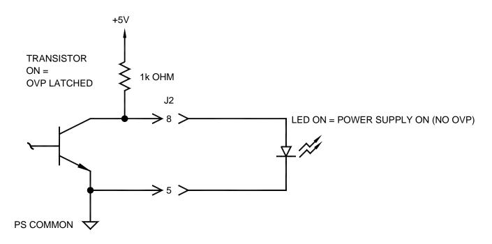
NOTE: NOT TO BE USED FOR SAFETY INDICATION FOR THE PRESENCE (OR LACK THERE OF) OF HIGH VOLTAGE
