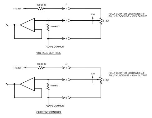
**Figure 3.2B Remote Programming Via External Resistance**
