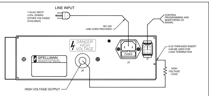
Figure 3.1 Typical Operating Set Up
