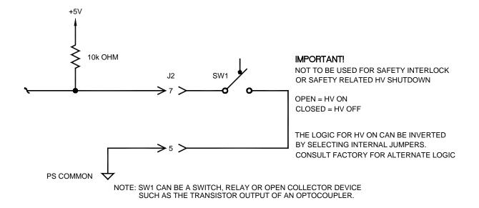
Figure 3.4 HV ON/OFF Control
