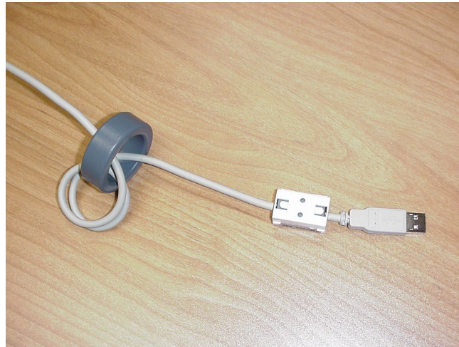
Figure 10 - Example of a USB Cable Using Ferrites
