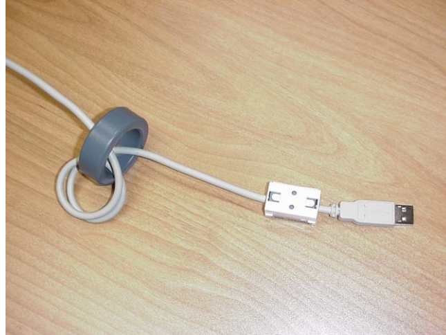
Figure 8 - Example of a USB Cable Using Ferrites
