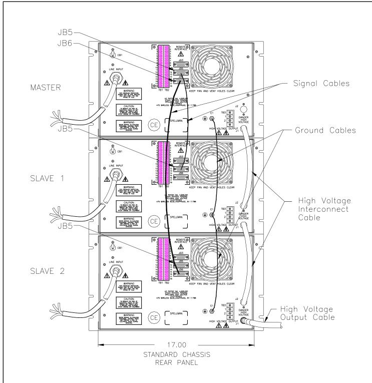
Figure 5.6 18kW Installation Drawing
