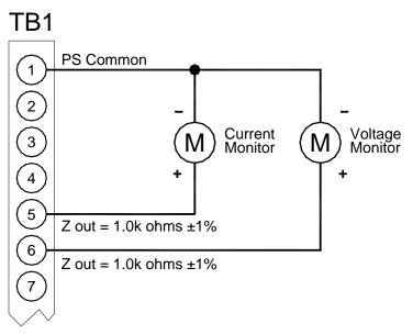
Figure 3.3 Remote Monitor Test Point Designations
