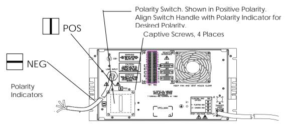
Figure 5.7 Rear Panel Polarity Reversal Switch
