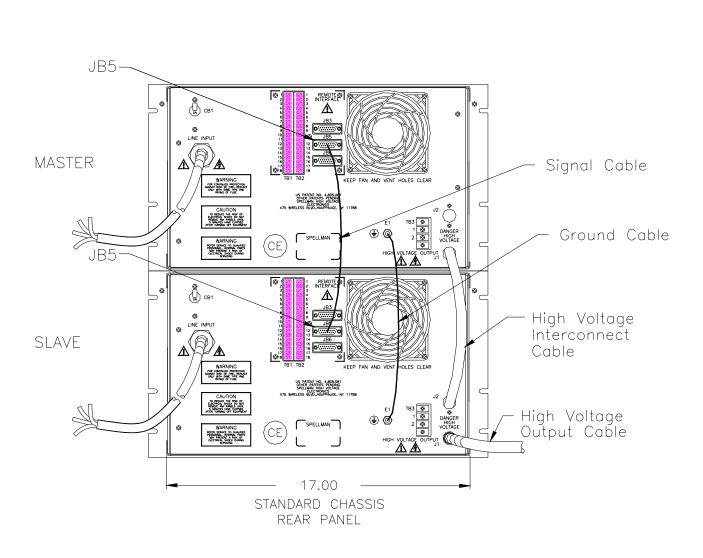
Figure 5.5 12kW Installation Drawing
