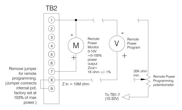
Figure 5.4 Adjustable Power Remote Interface
