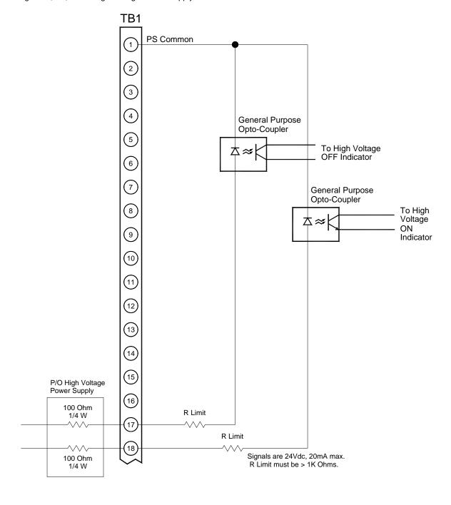
Figure 3.7 Remote High Voltage ON and Remote High Voltage OFF Indicator
