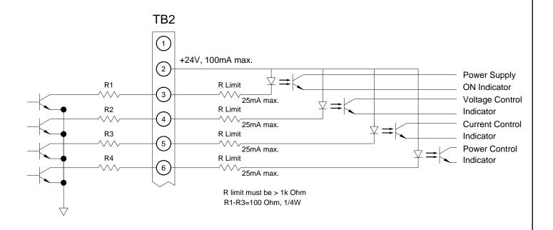
**Figure 5.2 Remote Mode Indicators Interface**
