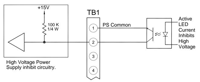
Figure 3.5 External Inhibit Interface Circuit
