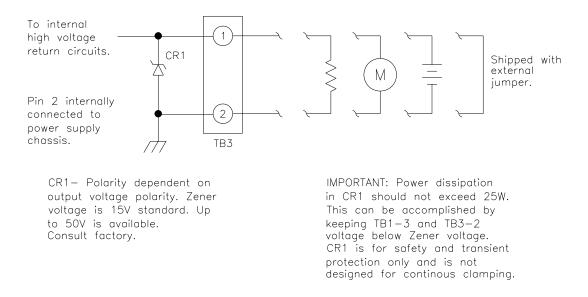
Figure 5.3 Floating Ground Interface Circuit
