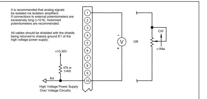
Figure 5.1 Remote Overvoltage Adjust Interface
