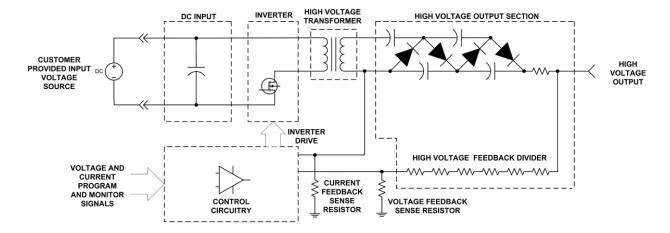
Figure 9 - Block Diagram
