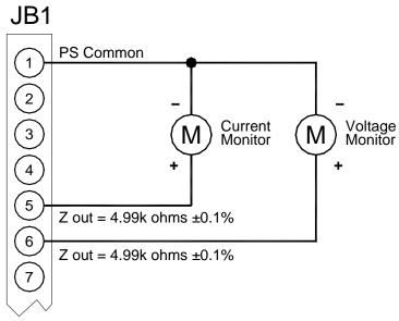
**Figure 3.4 Remote Monitor Test Point Designations**
