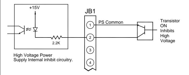
Figure 3.6 External Inhibit Interface Circuit
