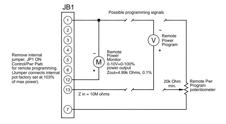
Figure 5.2 Adjustable Power Remote Interface
