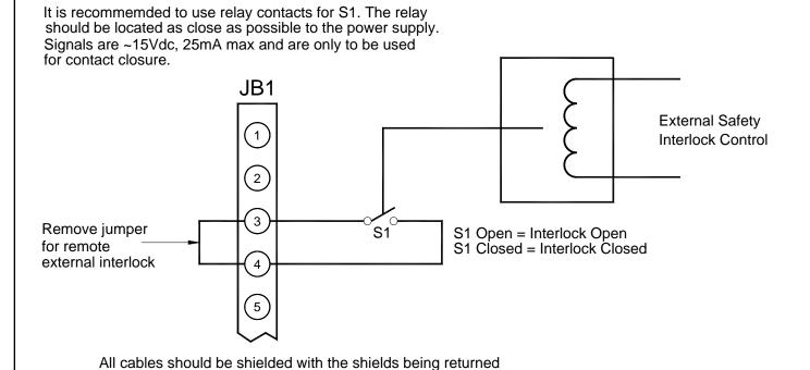
Figure 3.7 External Interlock Interface
