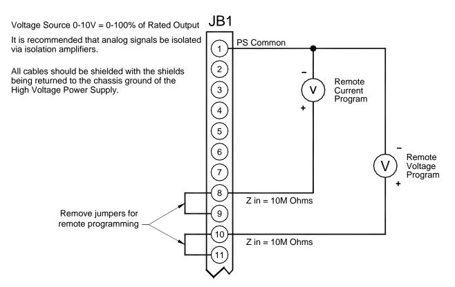
Figure 3.3A Wiring Diagram for Remote Programming Via Voltage Source
