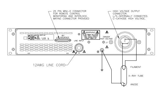
Figure 3.2 Typical Operating Setup XLF
