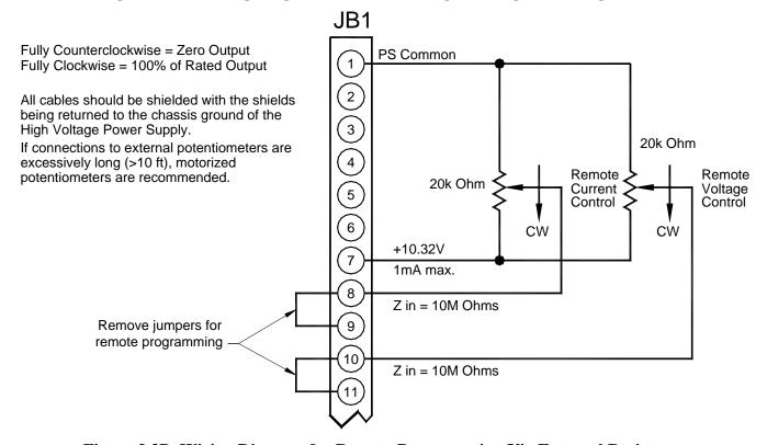
Figure 3.3B Wiring Diagram for Remote Programming Via External Resistance
