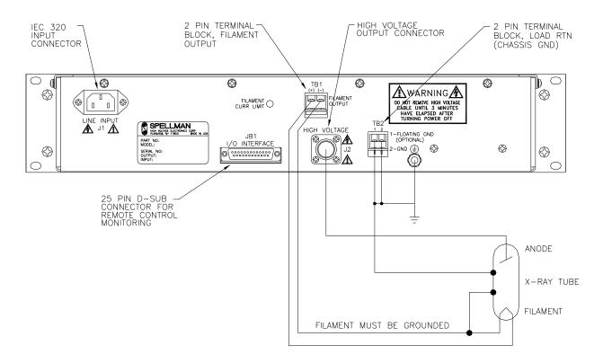
Figure 3.1 Typical Operating Setup XLG
