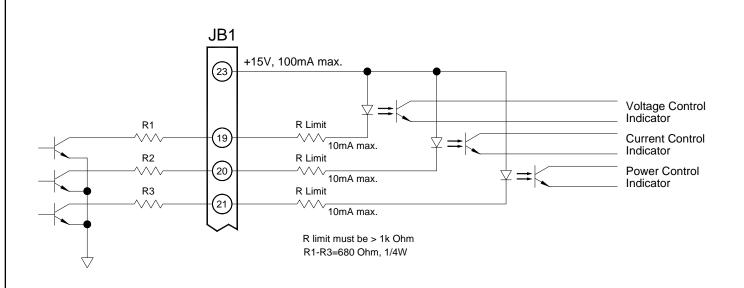
**Figure 3.9 Remote Mode Indicators Interface**
