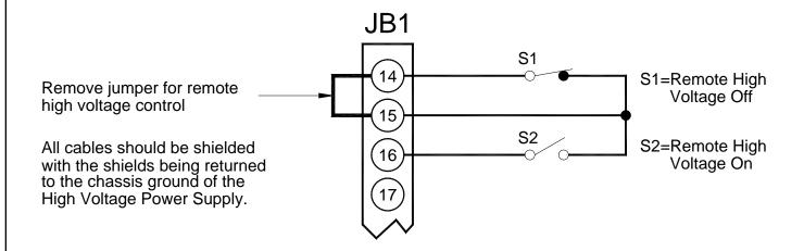
Figure 3.5 Remote Control of High Voltage ON and High Voltage OFF Interface
