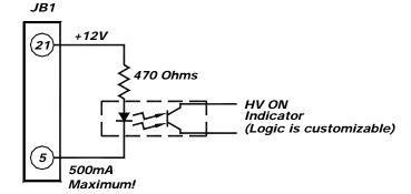
12dc lamps or relay coils may replace opto-couplers. Opto-couplers, lamps or relays should be located as close as possible to the high voltage power supply. All cables should be shielded with the shields being returned to chassis ground of the High Voltage Power Supply.
