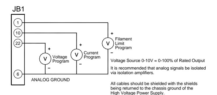
Figure 3.2A Wiring Diagram for Programming via Voltage Source
