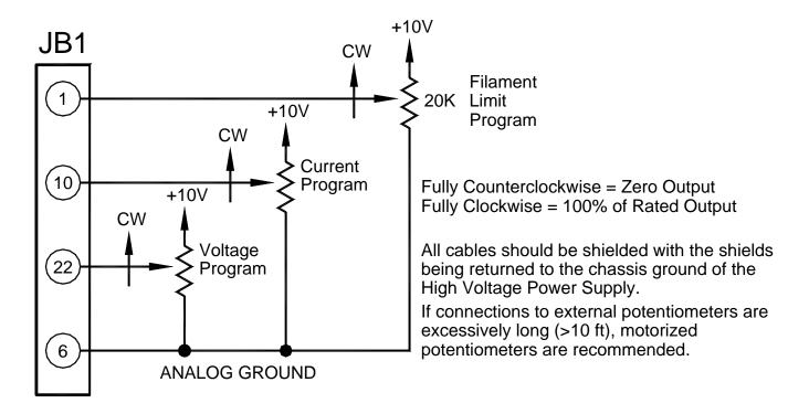
Figure 3.2B Wiring Diagram for Programming via External Resistance
