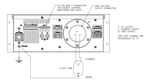
Figure 3.1 Typical Operating Setup XRF
