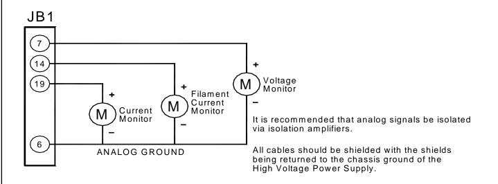
**Figure 3.3 Monitor Test Point Designations**
