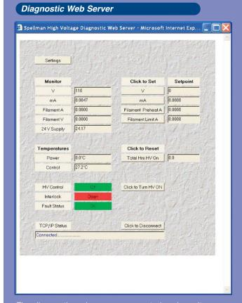
The diagnostic web server can control and monitor an SIC equipped power supply from a web browser It displays operating status of the Power Supply and allows the unit to be configured in real time. The application consists of three web pages; a page displaying contact information, a license agreement and a monitoring and control applet that is at the heart of this application
